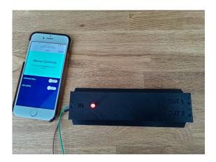
To demonstrate that ClearVue glass is producing power when providing sample products to third parties/customers, a new PCB has been designed with a Wi-Fi control interface. Potential clients can simply place the sample they have received into sunlight and connect to the Wi-Fi hotspot that has been established by the controller.
