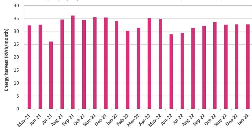
Monthly output (Array F, 12 windows on north wall, Murdoch University Solar Greenhouse)
