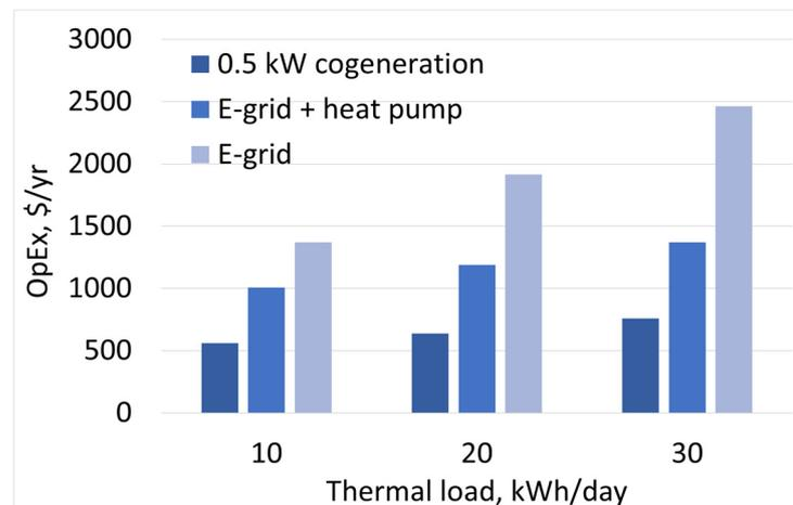
**Figure 9.** Annual operational expenditure of different system configurations with variable thermal loads: 0.5 kW cogeneration system at 40% electrical efficiency (2 kWh EES), heat pump with COP 3.0, and baseline electrical grid supported heating system (COP = 1.0); 15 kWh/day of electrical load, no PV.
