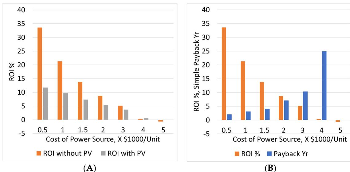
**Figure 8.** Economic analysis of the cogeneration system. (A) Influence of cost on ROI, with and without PV. (B) Payback period at different cogeneration system costs (no PV).
