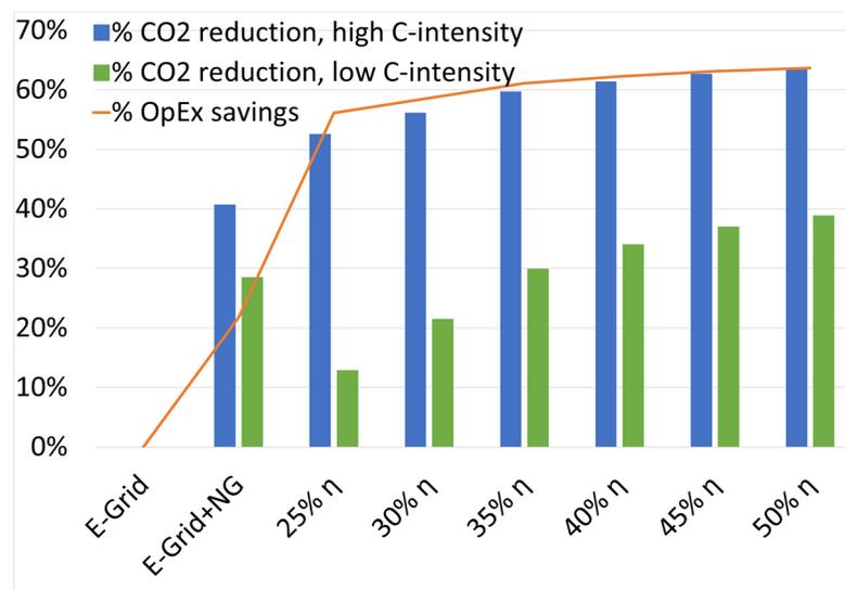
**Figure 7.** Environmental and economic analysis of cogeneration system-based configurations with different electrical efficiencies. Combined load of 28 kWh/day, 0.5 kW PV, 0.4 kW PM, and 2 kWh electrical storage capacitance.
