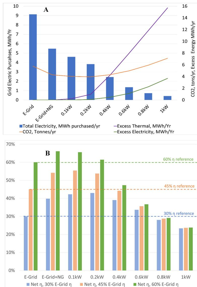
**Figure 3.** Influence of generator power scale on E-Grid demand, total carbon dioxide emissions, excess electrical and thermal energy produced, and net combined efficiency of the residential energy system. (A) CO<sub>2</sub>, E-Grid purchases vs. different configurations. (B) Total energy efficiency vs. cogeneration system power rating. No PV or thermal energy storage in the cogeneration system configuration.
