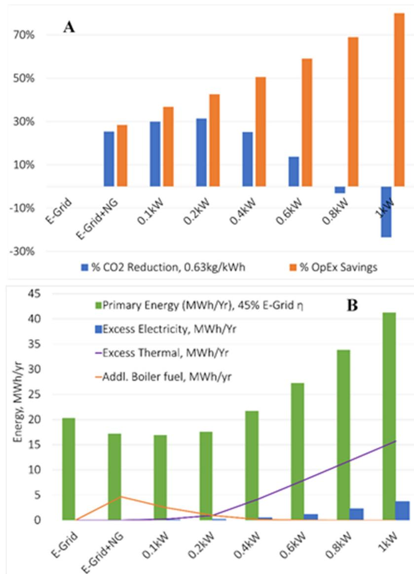
**Figure 4.** Impact of energy source configuration on carbon dioxide emissions, operational expenditure, primary energy consumption, heating fuel demand. (A) Reduction in CO<sub>2</sub> and operational expenses. (B) Total primary energy and additional heating fuel consumption. No PV in the cogeneration system configuration.
