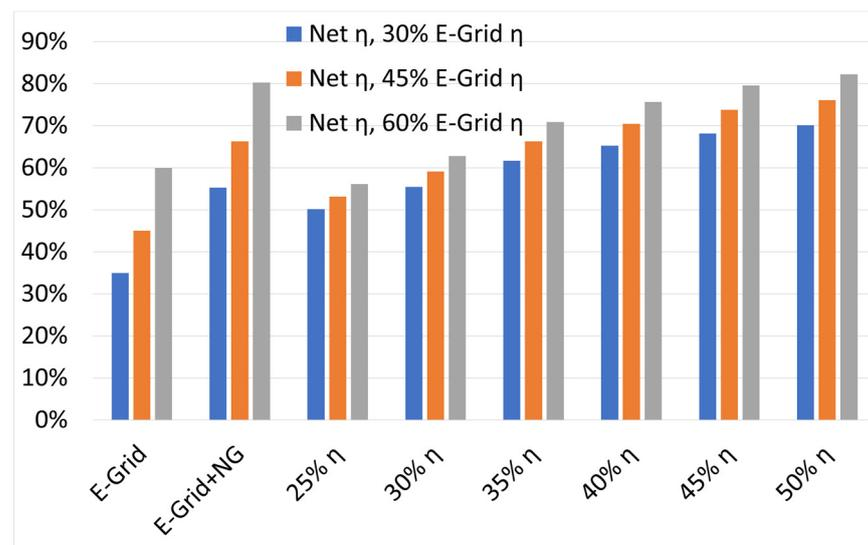
**Figure 6.** Combined energy efficiency of cogeneration system-based configurations with different prime power electrical efficiencies. Combined load of 28 kWh/day, 0.5 kW PV, 0.4 kW PM, and 2 kWh electrical storage capacitance.
