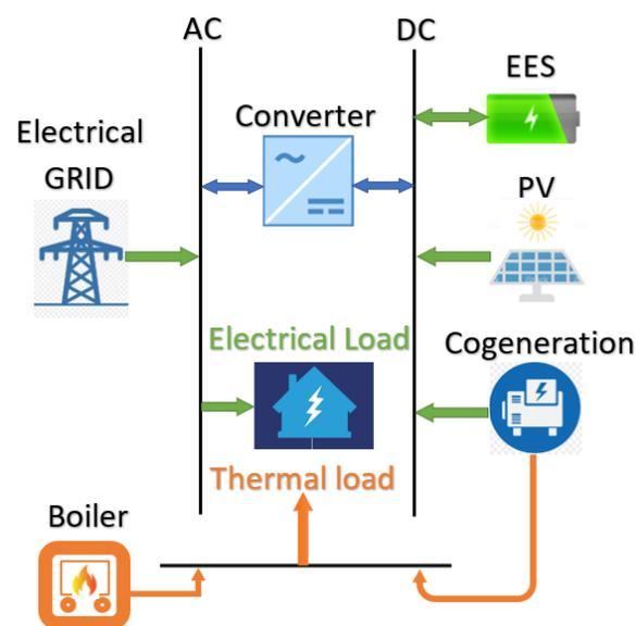
**Figure 2.** Generic hybrid energy system configuration utilized in this study.
