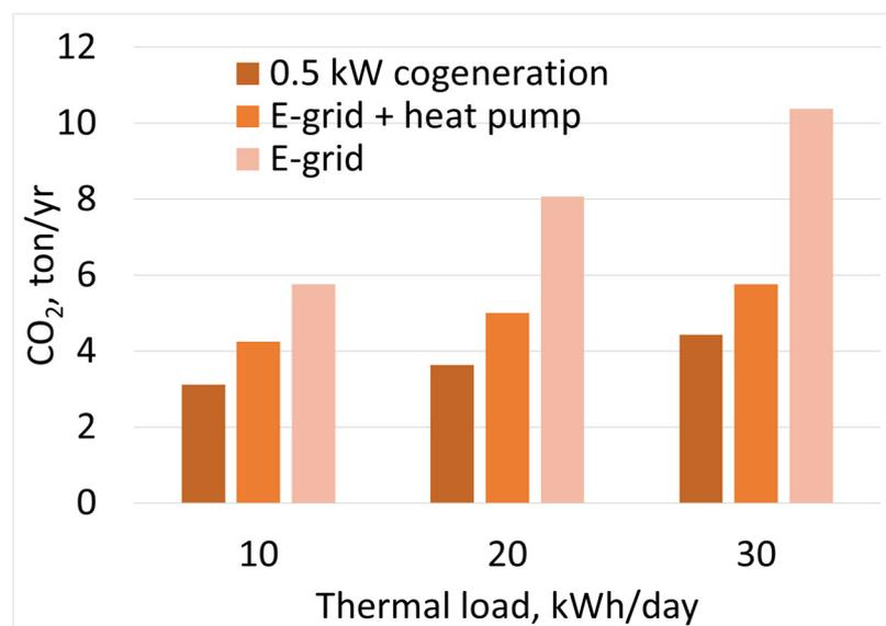
**Figure 10.** Annual carbon dioxide emissions of different system configurations with variable thermal loads: 0.5 kW cogeneration system at 40% electrical efficiency (2 kWh EES), heat pump with COP 3.0, and baseline electrical grid supported heating system (COP = 1.0); 15 kWh/day of electrical load, no PV.
