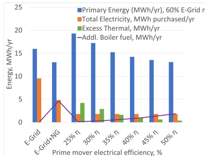
**Figure 5.** Energy performance analysis of cogeneration system-based configurations with different prime power electrical efficiencies. Combined load of 28 kWh/day, 0.5 kW PV, 0.4 kW PM, and 2 kWh electrical storage capacitance.
