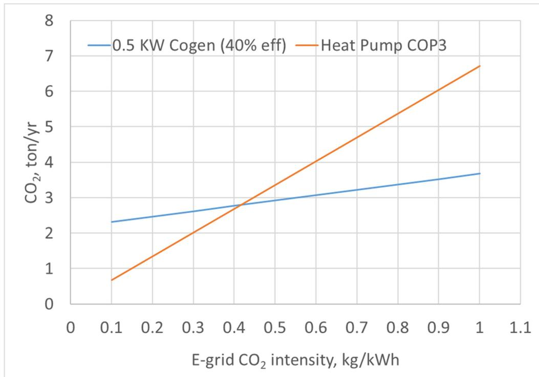
**Figure 11.** Annual carbon dioxide emissions of a residential building served by a 0.5 kW cogeneration system (40% electrical efficiency) or E-grid-supported heat pump system (COP-3).
