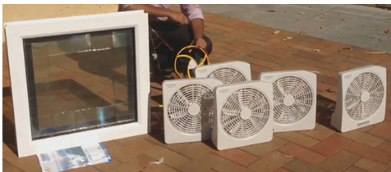
Figure S5. Powering household appliances. A 500mm x 500mm framed microstructured-glass concentrator during outdoor performance testing in May 2015. All five of the series-connected DC fan systems were able to run simultaneously at an appreciable rotation rate when powered by the sample.
