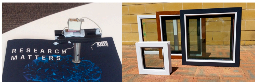
Figure 6. Solar window prototypes developed at Edith Cowan University (ECU between 2011–2016).
