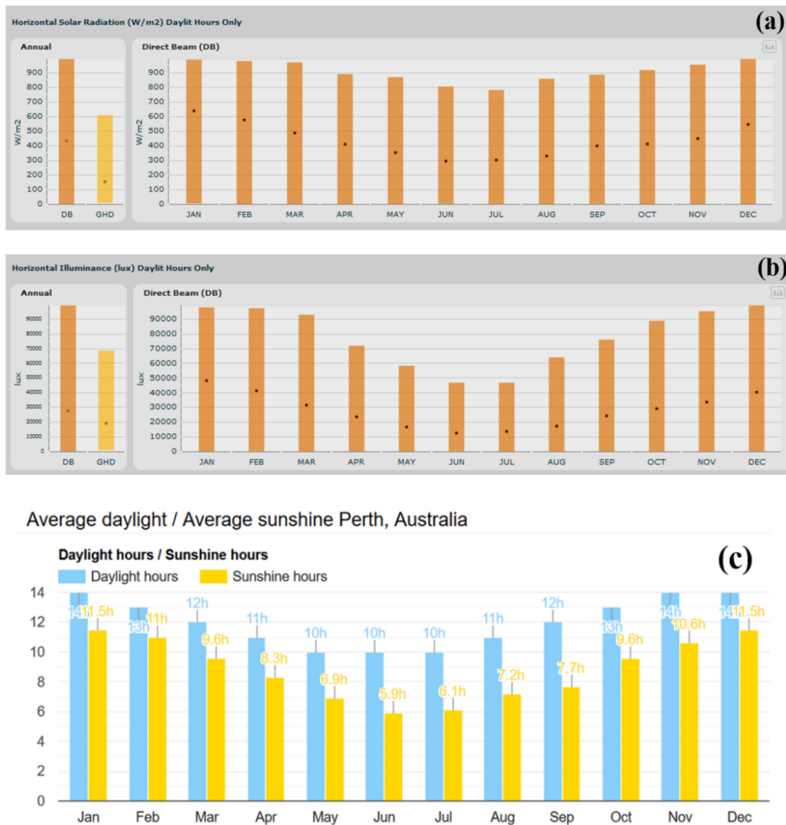
Figure 7. Seasonal yearly climate-related solar irradiation parameter variations for Perth, Australia. (a) Monthly averaged and maximum-recorded direct-beam solar irradiation intensities measured across horizontal plane; (b) monthly averaged and maximum-recorded direct-beam solar illuminance values measured across horizontal plane; (c) monthly distributions of the total daylight hours and the daily sunshine durations. The datasets shown in parts (a) and (b) have been obtained using COMFEN 5 software [46]; the dataset of part (c) has been published online by [31], using the publicly-available Australian Bureau of Meteorology data.
