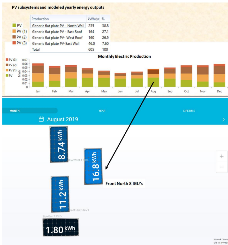
Figure 3. A summary of the predicted monthly and yearly microgrid energy output results modeled using HOMER Pro software package; the measured electric energy generation amounts during the month of August 2019 are also shown (data obtained from the Enphase Enlighten™ monitoring software records).
