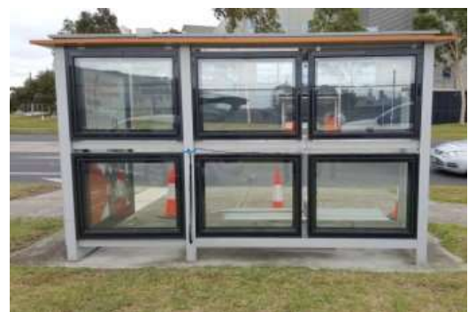
PHOTO: The energy harvesting solar-glass has been trialled as a self-sustainable bus shelter in Melbourne. (Supplied: Victor Rosenberg)
